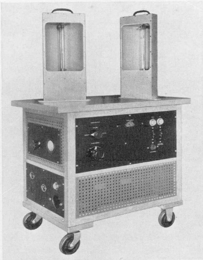
FIGURE 2. Control unit of the TYPE 621-H Edgerton Power Stroboscope showing the mercury lamps. The complete stroboscope consists of this unit and a 10-kw motor generator
